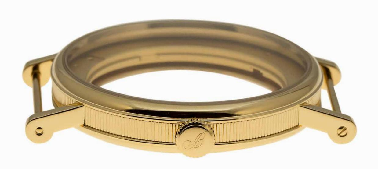
The case back is pushed onto the centre of the case and sandwiches in place a silicone seal assuring the watch remains water resistant. To remove the caseback with out damaging the flooting on the vertical section of the case centre, a knife edged blade is used at a specific point at 9 oclock to lever the case back off.
